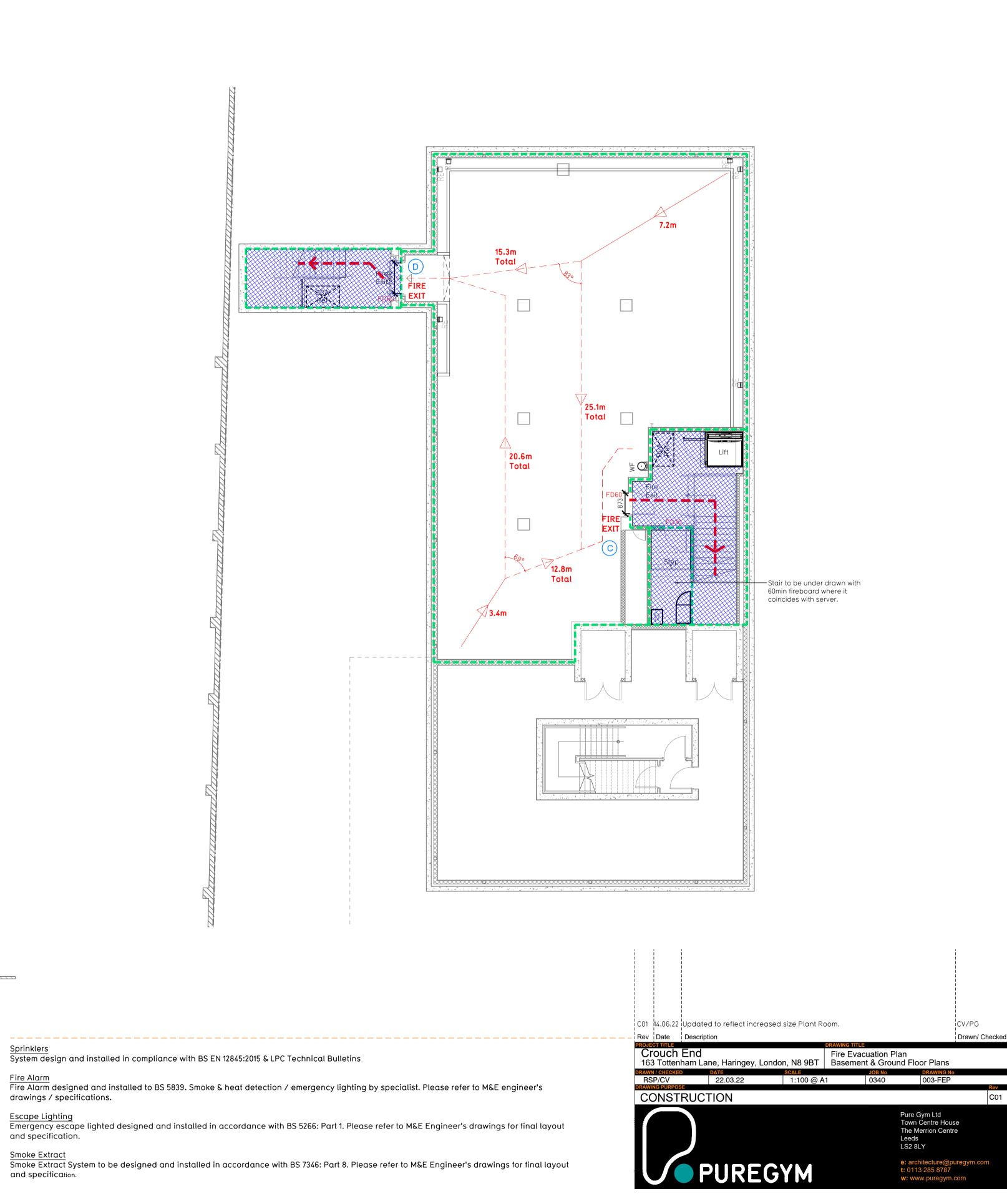
Escape Lighting Emergency escape lighted designed and installed in accordance with BS 5266: Part 1. Please refer to M&E Engineer's drawings for final layout and specification.
