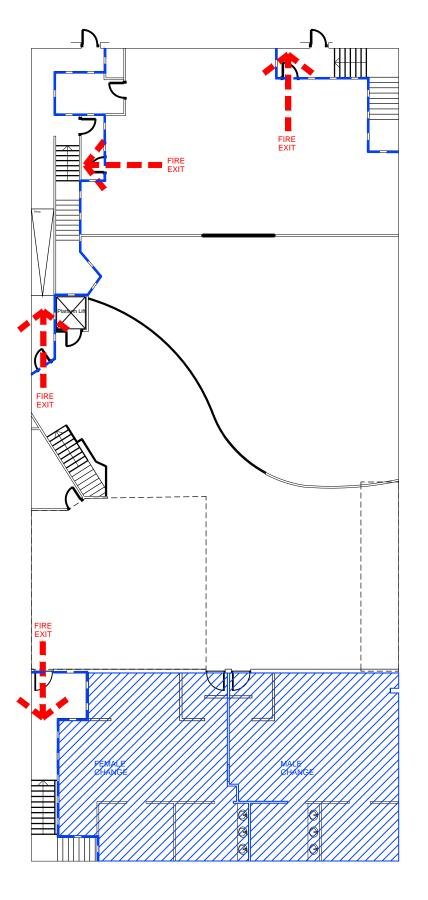
DENOTES 60min FIRE RATED COMPARTMENT WALLS WITH 30min FIRE RATED DOORS
